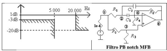
$R_1 = R_3 = 18,969 \text{ k}\Omega$   $R_2 = 431,162 \text{ k}\Omega$   $R_4 = 1,742 \text{ k}\Omega$   $R_5 = 39,607 \text{ k}\Omega$   $C_1 = C_2 = 1 \text{ n}F$  $R_{P1} = R_{P2} = 3,183 \text{M}\Omega$
